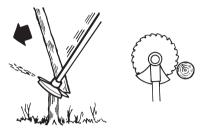
To fell to the right, the bottom of the tree should be pushed to the left. Tilt the blade and bring it diagonally up to the right. Cut with the area of the blade between 3 o'clock and 5 o'clock so that the direction of rotation of the blade pushes the bottom of the tree to the left.
