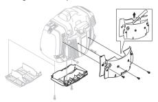
IMPORTANT! The machine MUST be returned to its standard design at temperatures warmer than 5°C. Otherwise there is a risk of overheating resulting in serious engine damage.
