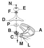
Screw the support cup (E) onto the output shaft threads (CAUTION! Left-hand thread). Tighten to a torque of 35-50 Nm (3.5-5.0 kpm). Use the socket spanner in the tool kit. Note that the locking pin (C) must remain inside the gear housing to lock the drive disk. Hold the shaft of the socket spanner as close to the blade quard/combination quard as possible.
