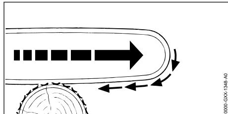
The saw is pulled away from the operator when the bottom of the bar is used for cutting.
