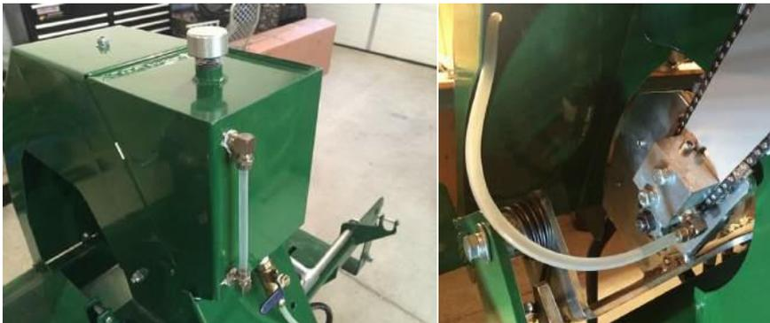
9. Install the back plate, reinforcement bracket, and the top pulley housing to the chainsaw bar guard using the bolts provided. Tighten all bolts including the bolts from step 7.
