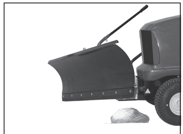
4) The angle setting mechanism is released and the shovel blade clears the obstacle.
