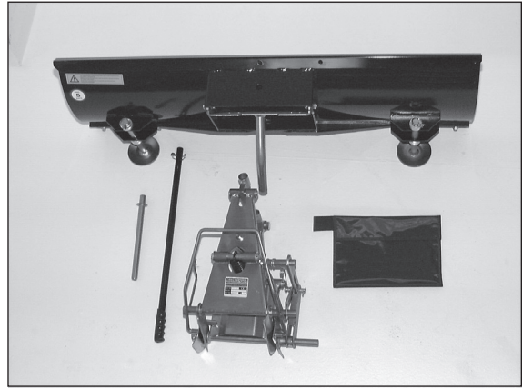
Specifications of shovel blade attachment
