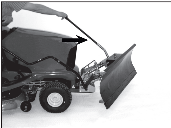
3) Lift the operating rod and turn the shovel blade to the desired angle.
