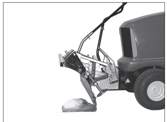
2) Shovel blade lower edge folds back. Safety folding mechanism disengaged.
