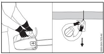
If kickback occurs, the saw can be thrown up in the direction of the operator. Due to the special handle design (closely spaced handles) there is a risk of the operator losing control of the chainsaw and sustaining serious or fatal injuries. Hold the saw firmly with both hands.
