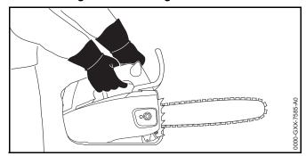
► Hold and control your saw with your left hand on the handlebar and your right hand on the top handle. Wrap thumb of left hand around the handlebar and thumb of right hand around the top handle.
