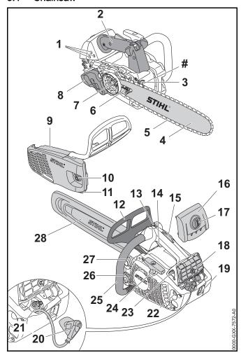
1 Carburetor Adjusting Screws For tuning the carburetor.
