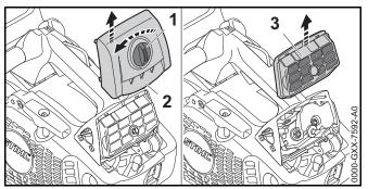
► Rotate the shroud lock (1) a half turn counterclockwise.
