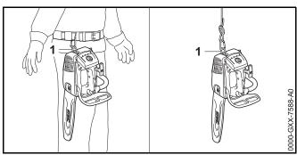
The chainsaw can be carried by attaching the ring (1) to your waist belt or a rope.
