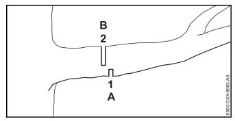
Make a relieving cut (1) in the compression side (A) first, then perform bucking cut (2), offset in direction of trunk, at the tension side (B).
