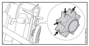
If there are visible wear marks: Do not use the chainsaw and contact your STIHL servicing dealer for assistance. The chain sprocket must be replaced.
