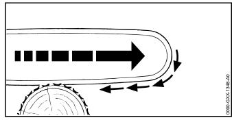
The saw is pulled away from the operator when the bottom of the bar is used for cutting.
